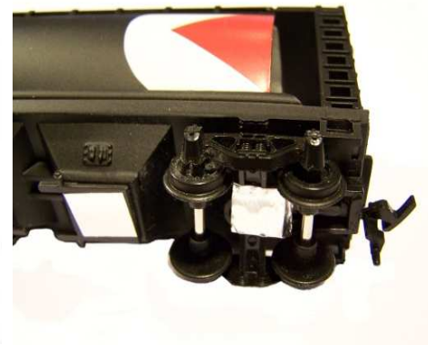
Cut into cubes and stick to underside of rolling stock.
